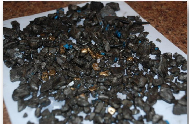
Debris sample, stage tool millout.
